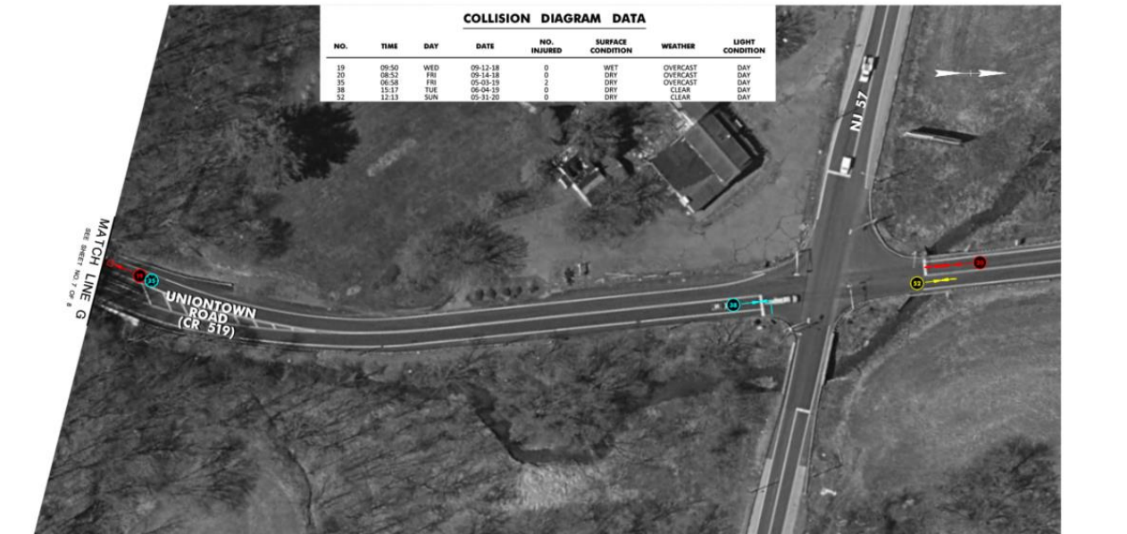
Figure 10: 519 Roadway Safety Audit Collision Diagrams
