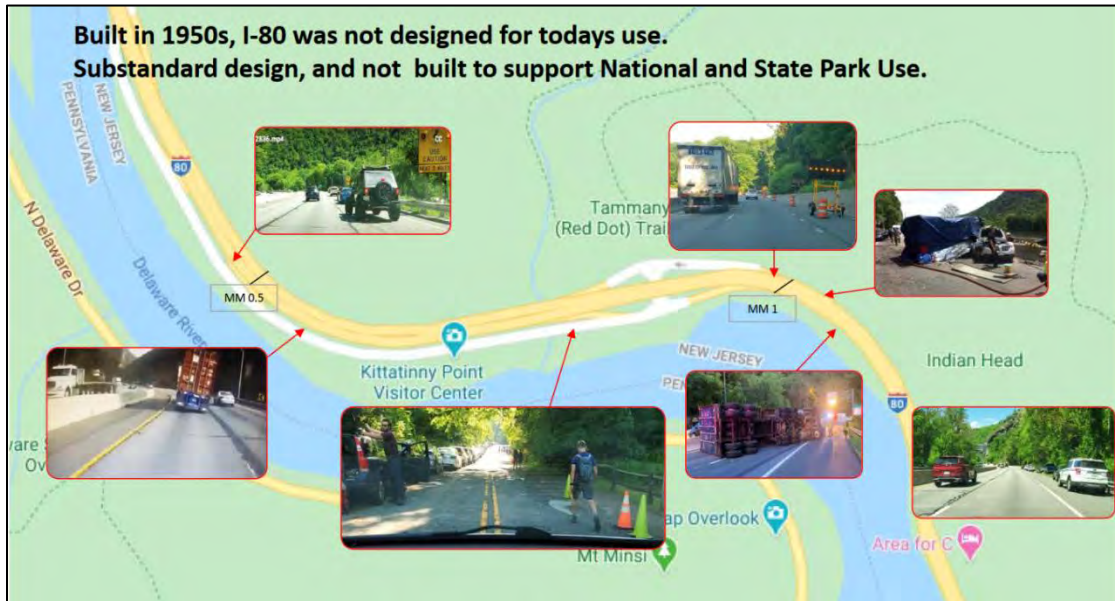
Graphic from NJDOT Problem Statement Identifying Design Deficiencies
